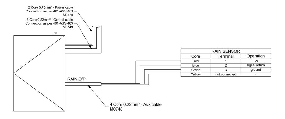
\*\*Cables exit from the underside refer to kerb drawing 401-ASS-401 for detailed exit position
