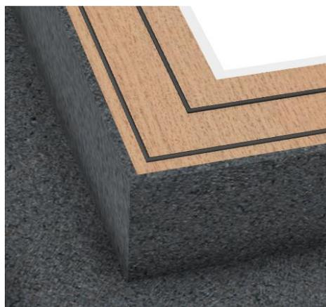
*Figure 5 - Silicone placement*
