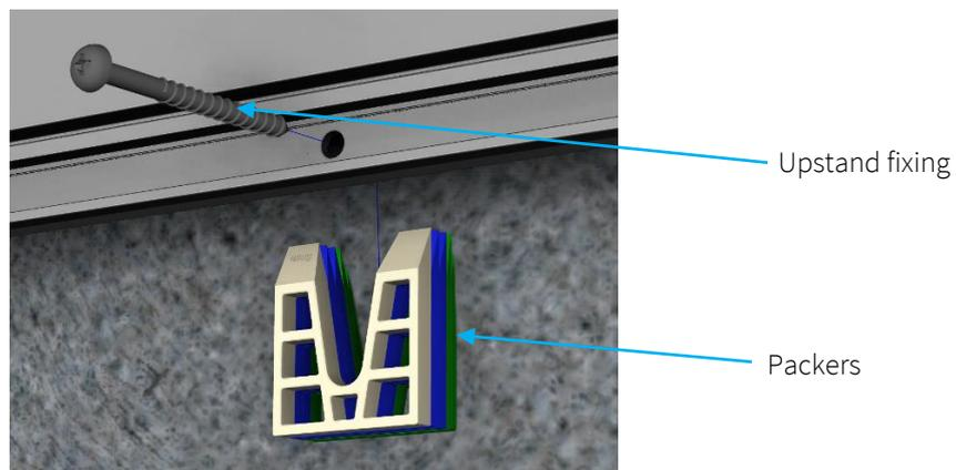
Figure 6 - Upstand fixings
