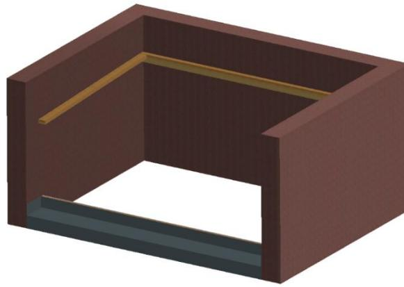
Figure 2 - Temporary wooden support battens in place
