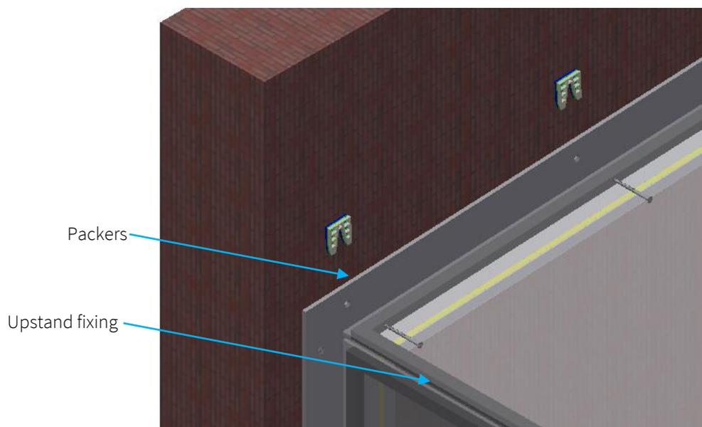
Figure 3 – Wall fixings
